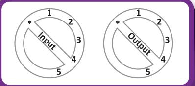
The input dial controls how much heat is stored overnight. The higher the number you set it to, the more heat is stored. The output controls how quickly the heat is released. The higher the number you set it to, the quicker it releases the heat.
